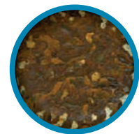
Galvanized Z275 after 1440 hours of salt spray testing.
